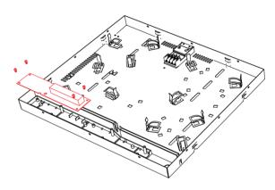
Step 5: remove the power board
