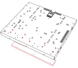
Step 6: to remove the display board fixing box, reverse the base and remove the screws
