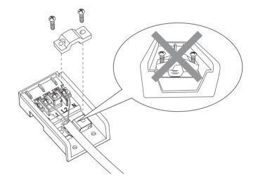
5. Assemble the cable clamp, be aware that the ellipse hole on cable clamp must match the ellipse hole on.
