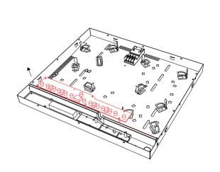
Step 4: remove the display board
