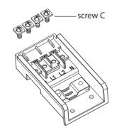
4. Remove the 4 screws C in the terminal box and insert the power cord at the connection.
