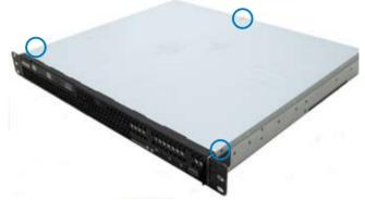
2. Firmly hold the cover and slide it toward the rear panel for about half an inch until it is disengaged from the chassis.
