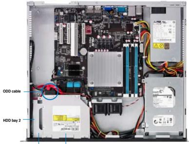
HDD drive tray Optical Disc Drive
