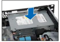
Secure the HDD drive tray and the 3.5-inch SATA HDD assembly to the HDD bay 2 using the four screws removed in step 2
