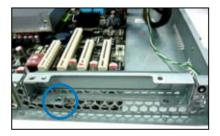
Remove one more screw to release the metal slot cover from the expansion card bracket.
