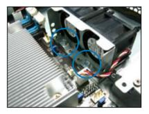
Connect the chassis fan cables to the onboard fan connectors labeled FRNT\_FAN2, and FRNT\_FAN3.
