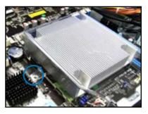
3. Replace the screw and secure the airduct onto the motherboard.
