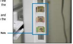
5. Adjust the length of the outer rail to fit the length of the rack cabinet, then fasten the two screws.
