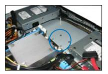
Position the chassis fans to match the screw holes on the chassis. Secure the fans onto the chassis using the provided screws.
