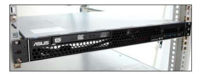
Secure the server to the rack with one rack screw at one side. Secure the other side as well.
