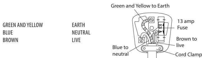
As the colours of the wires in the mains lead of this appliance may not correspond with the coloured markings identifying the terminals in your plug, proceed as follows:
