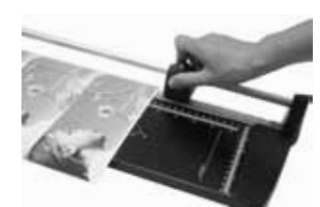
3. Slide the rotary blade across the bar to cut paper.
