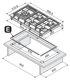
Carefully position the supplied insulating seal **(E)** on the outer perimeter of the hole made in the counter top, trying to make it stick on the entire surface by applying light pressure on it with your hands. Once the hob is fixed in position remove excess material using a cutter.
