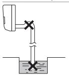
• Drain hose extension. To extend the drain hose, use a field supplied hose with inner Ø16 mm. Do NOT forget to use a heat insulation tube on the indoor section of the extension hose.
