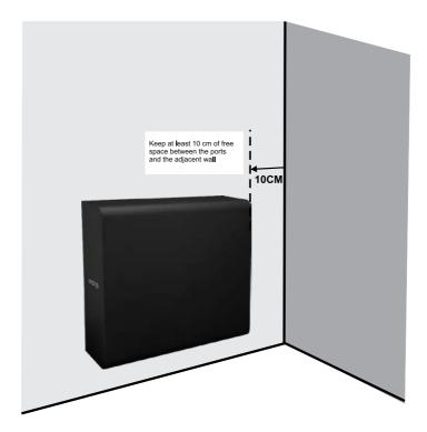
Do not block the bassports at the side of the speaker. Keep at least 10 cm of free space between the ports and the adjacent wall
