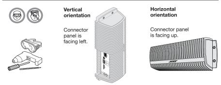
Follow these instructions to wall mount your SoundTouch<sup>TM</sup> SA-4 amplifier. Install either vertically with the connector panel facing left, or horizontally with the connector panel facing up.
