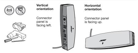
Follow these instructions to wall mount your SoundTouch<sup>™</sup> wireless adapter. Install either vertically with the connector panel facing left, or horizontally with the connector panel facing up.
