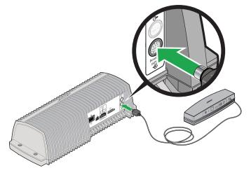
**4.** When prompted by the app, plug the power cord into the **AC POWER** connector on the back of the SoundTouch<sup>™</sup> SA-4 amplifier.
