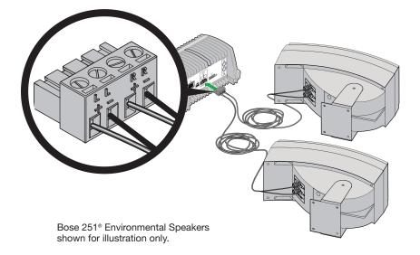
4. Plug the terminal block connector into the **SPEAKER OUTPUTS** connector.
