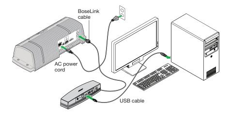
Note: Connect the USB cable to the SoundTouch<sup>™</sup> wireless adapter only when the app instructs you to do so.
