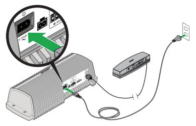
5. Plug the other end of the power cord into AC (mains) power.
